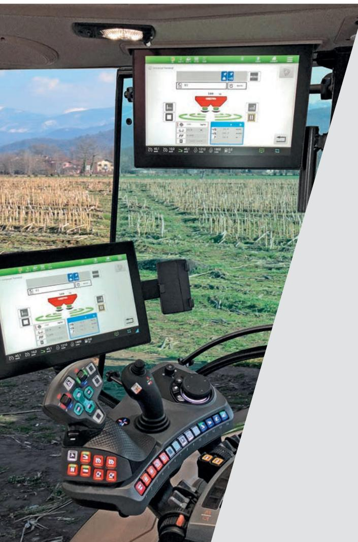
By connecting these types of fertilizer spreaders to a **ISOBUS** tractor / device, a simple and intuitive **Universal Terminal** for management the functions of the fertilizer spreader is displayed.
