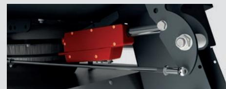
Two magnetic sensors detect the exact opening of each shutter and control directly the linear actuators avoiding any possible error of position.
